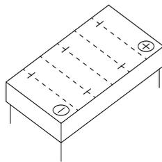
**Technology** Sealed maintenance-free AGM battery | electrolyte held in Absorbent Glass Mat separators | wet charged
