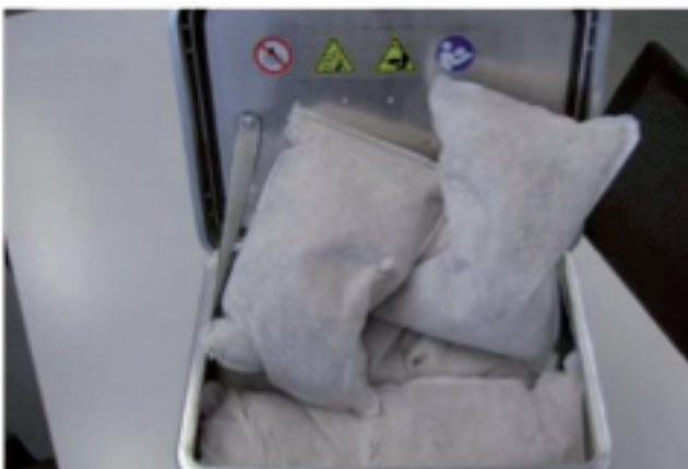
Thermal insulation material, e.g. Vermiculite
